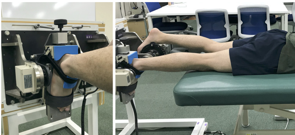
Figure 2. Measurement of torque during isometric ankle plantar flexion using a custom-made ankle joint torque meter. The subject lies prone on the bed. The foot is fixed to the foot plate by a strap, and the ankle joint angle was flexed at 0^\circ for ankle dorsiflexion. The subject is asked to exert force only to execute ankle plantar flexion during isometric contraction.
